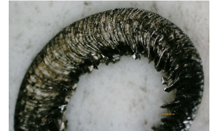
Lamellar chip flow, MR YG214 SS304
